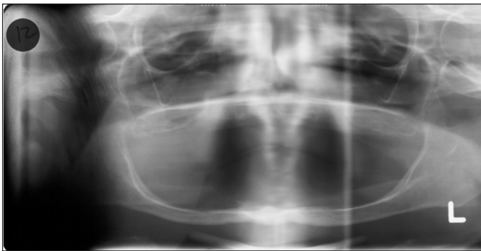
Figure 3 – Light leak from torn cassette
